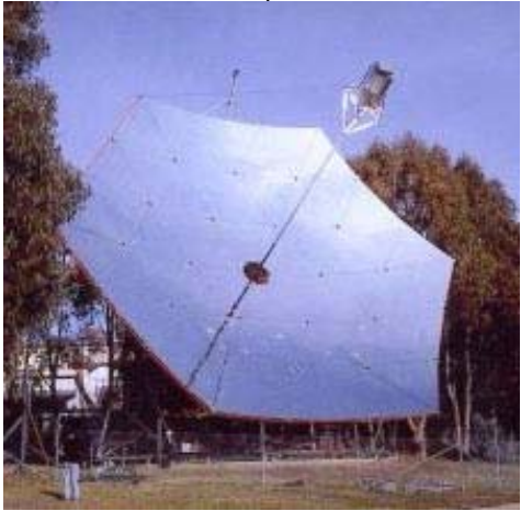
Figure 13. The 400m 2 SG3 dish prototype at the Australian National University.
